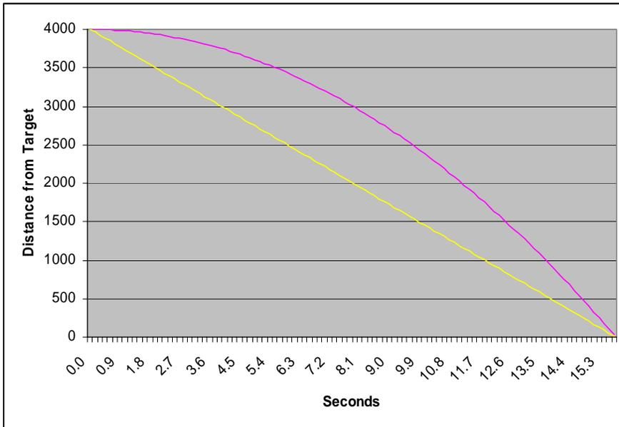
Car B competes with gravity only because it starts the trial having already attained its full velocity, while car A starts with a velocity of zero.
